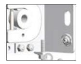
c. Finger tighten top nut. Leave approx. 6 threads exposed above nut.
