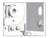
c. Finger tighten top nut. Leave approx. 6 threads exposed above nut.
