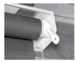
Set the housing into the groove at the top and bring down to set into place.
