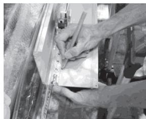
Using a 3/8" metal drill bit, drill the two mounting holes.
