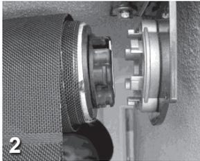
Reinstall motor clip onto bracket, making sure mouth snaps in place over bracket and motor head (#4,5).
