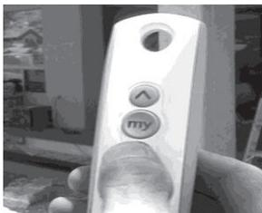
Run shade up and down a few times by pressing the up and down arrows on the provided remote to be sure there are no adjustments needed.
