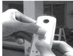
To change the lower limit, send the motor to its current lower limit by pressing the down arrow.
