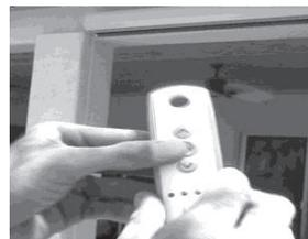
This saves your lower limit. To change the upper limit, send the motor to its current upper limit.
